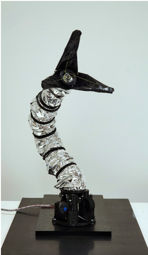
Figure 2: A soft robotic manipulator designed for extreme space conditions.
